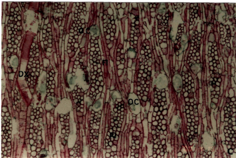
Tangential Longitudinal Section of Wood
