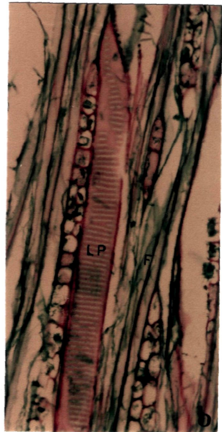
Tangential Longitudinal Section of Wood
