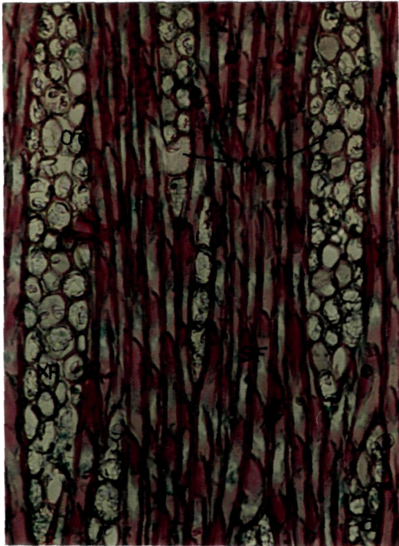
Tangential Longitudinal Section of Late Wood
