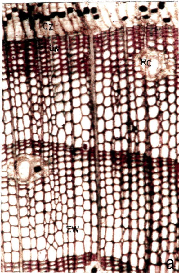
Transverse Section of Wood showing Distinct Annual Rings, Resin Canals
