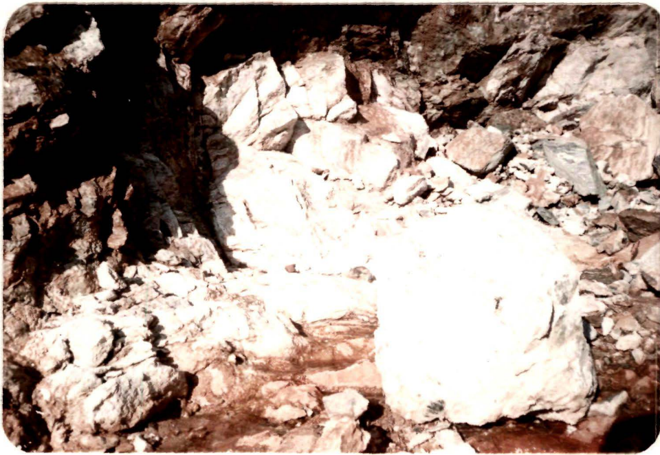
Plate No. 5 Sillimanite boulders (Open cast mining of Sillimanite at Sonapahar)
