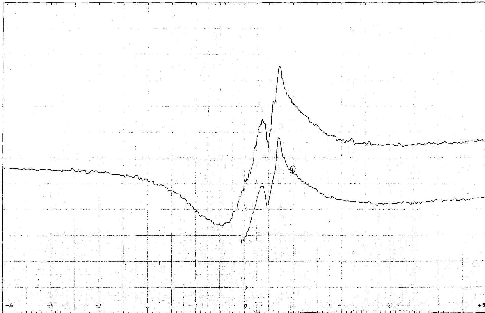
Fig. 5.4 (b) EPR spectrum of [\text{Cu}(\text{H}_2\text{slox})] ( 5.1 ) in DMSO at Temperature: RT; Frequency: 9.1 GHz; Scan Range: 2000 G; Field Set: 3200 G.
