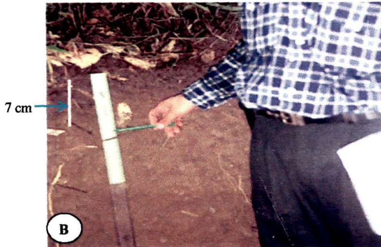
Soil profile of the MDF site with moderately thick layer of humus; average thickness of A_h horizon is 0-7 cm
