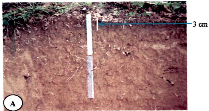
Soil profile of the DF site with very thin layer of humus; average thickness of A_h horizon is 0-3 cm
