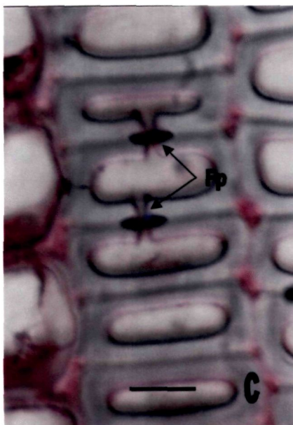
Transverse sections of wood showing inter fibres pits
