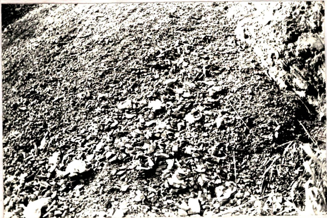
Disintegrated Sandstone of unequal size due to Mechanical weathering near Tuichawng village.
