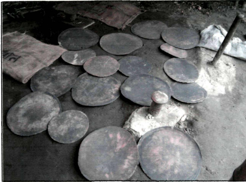
Plate 15 - Plate ready for moulding in to ' Taal ' (Cymbal)
