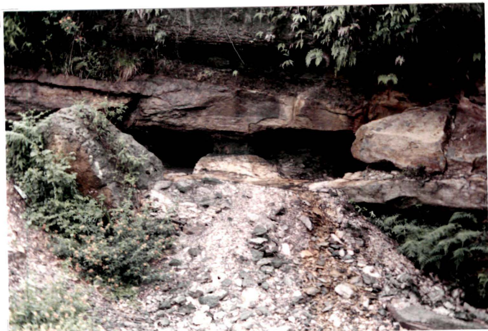
Plate 1.1B . Pit formed as a result of " rat hole" method of mining on the hill slope.
