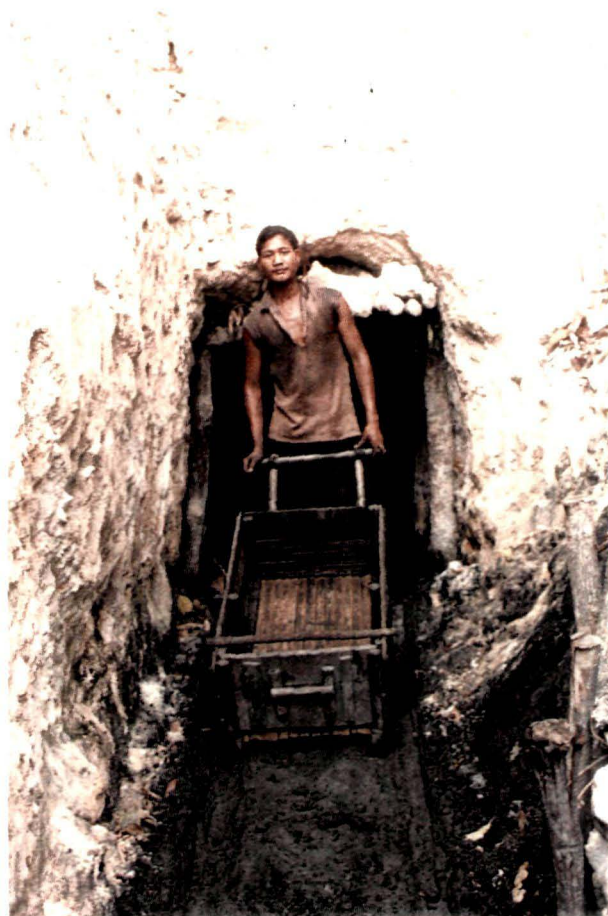
Plate 1 Coal mines in Nokrek Biosphere Reserve: The photographs showing the entry/exit path of the mines. Rat-hole mining method—a crude mining technique is the sole method of coal extraction in the Biosphere Reserve.
